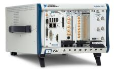
Figure 3. This PXI Express system includes the NI PXIe-8133 controller, which is capable of a maximum system bandwidth of 8 GB/s, as well as an NI high-speed digitizer.
