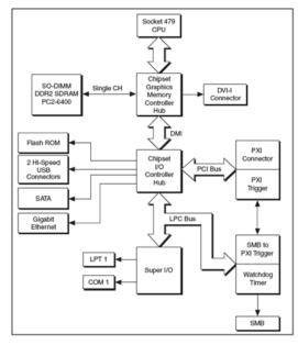
Figure 2. NI PXI-8101 Block Diagram
